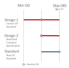
Design 1: The former GP standard had a nominal dimension of 6.906" with a plus/minus (+/-) tolerance. Maximum OD is 6.938".
